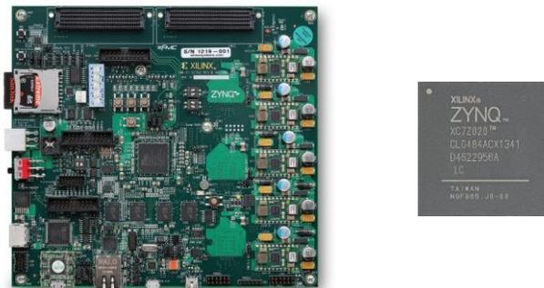
**Figure 3:** ZC702 board and ZC7020 Zynq chip
